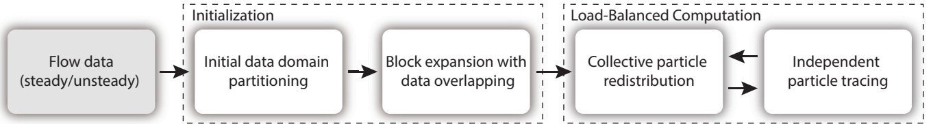
Fig. 2. Workflow of our load-balanced parallel particle tracing method. The raw flow data is first partitioned into blocks in the initialization stage. These blocks are further expanded by adding ghost layers on them to maximize the overlap with other blocks as much as possible. In the computation stage, collective particle redistribution and independent particle tracing are alternately executed to achieve load balance dynamically.
