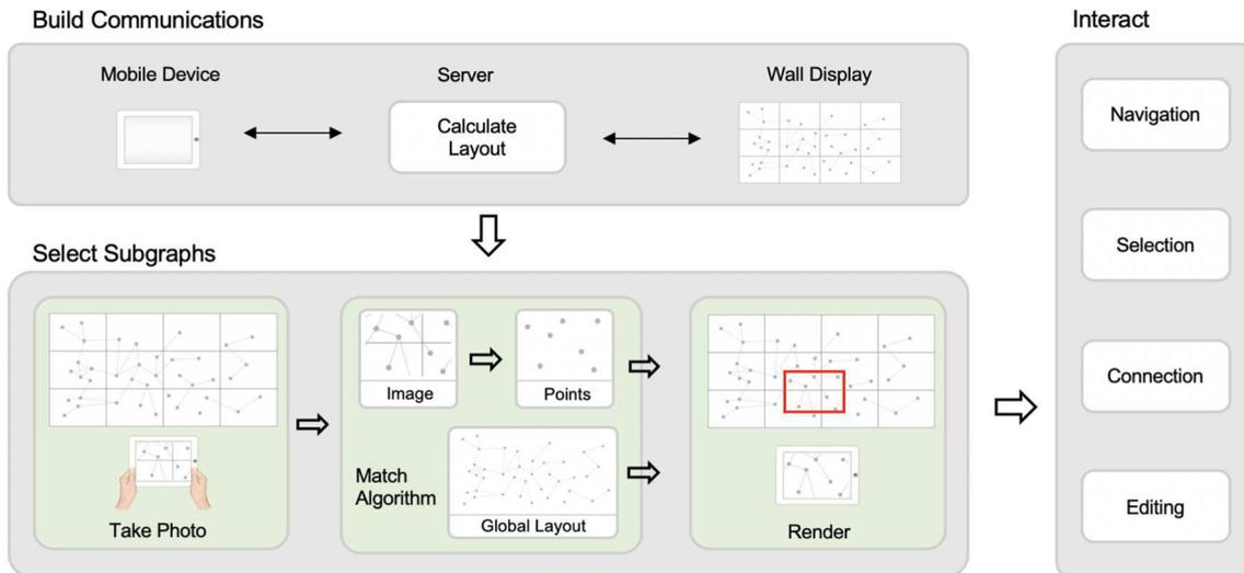
**Fig. 2** System overview. The system consists of three parts, visualization rendering on wall-sized display, local view selection by photoing, and interaction on display through the mobile device
