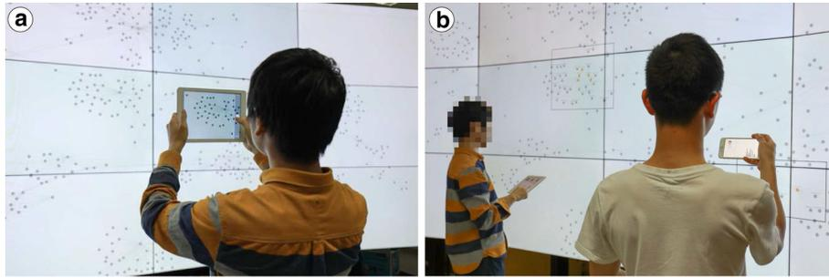
**Fig. 1** Photo4Action supports graph visualization exploration on the wall display through mobile devices. Users can take photo to select the subgraph (a) and explore details on mobile devices (b)
