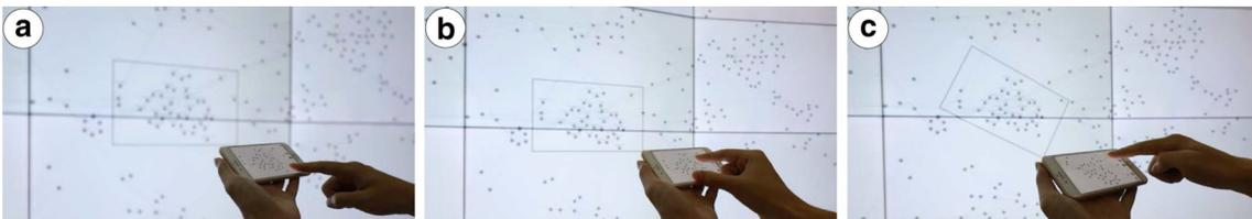
**Fig. 4** Users can pan, zoom, or rotate on the screen to further refine the focus area. **a** Fingers pan on the screen to move the selection area. **b** Two fingers pinch to zoom in/out the graph. **c** Extra widget is provided to rotate the focus
