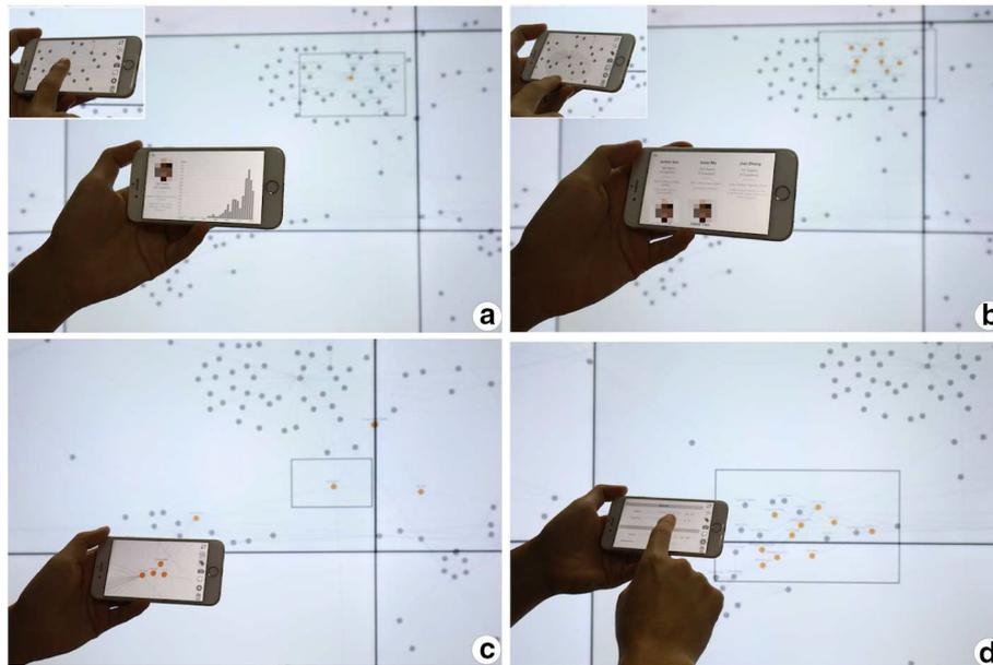
**Fig. 5** Different types of selection methods are supported. **a** Tap a node and show its details; **b** Select a group of nodes by lasso; **c** Select neighbors of nodes; **d** Select nodes within the data range
